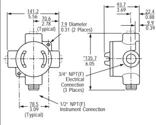
\*Dimension shown is approximate and based on a 5-thread engangement.
